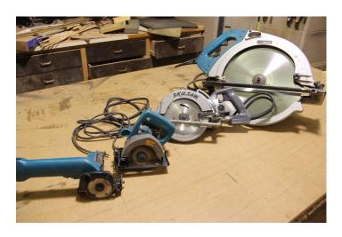
I have, due to my occupation, over time, collected an assortment of skill saws. The smallest has a 3 inch blade, then we step up to one with a  $4\frac{1}{2}$  inch blade. Next in line would be a  $7\frac{1}{4}$  inch version. The largest, is a big step up. It is a whopping 16 inch saw.
